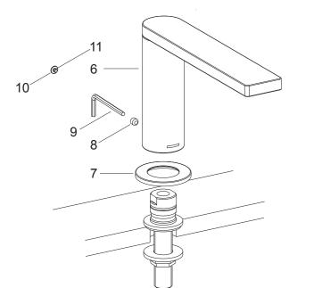
Remove the plug(10) with o-ring(11) in the back of spout. Loosen the screw(8) by hex wrench(9).
